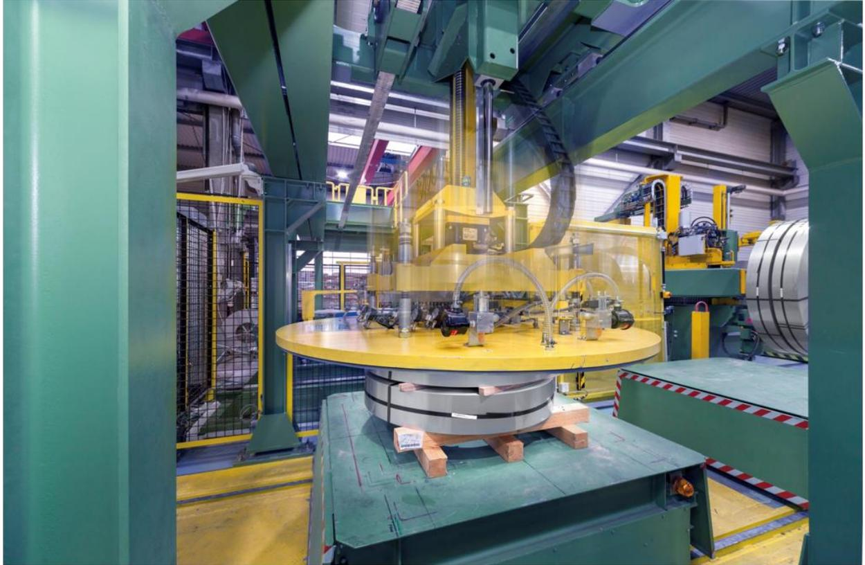
*The braking energy generated when lowering the load is stored on an interim basis with a KCM module from KOLLMORGEN.*
